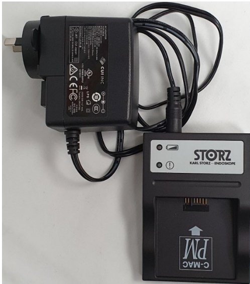
Fig 3: Battery charging station
