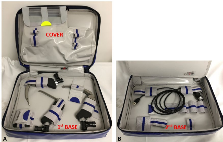
A: Cover holds C-MAC® pocket monitor. 1 st base holds battery and Miller 1, MAC 2, MAC 3 VLs with protective caps attached B: 2 nd base holds video connection cable
