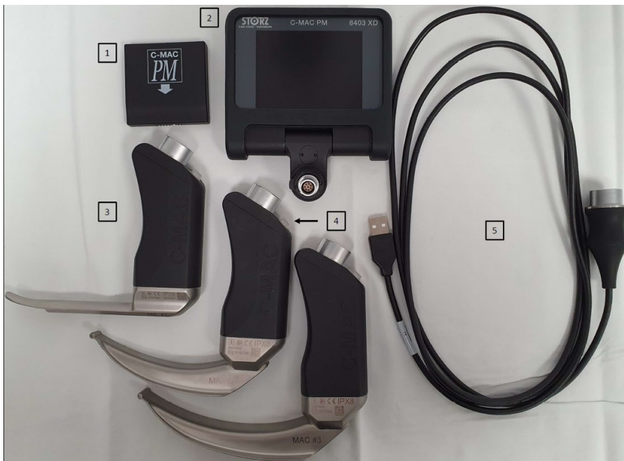
Fig 2: 1. Battery 2. C-MAC® pocket monitor 3. Laryngoscope blades (Miller 1, MAC 2, MAC 3) 4. Multifunctional button 5. Video connection cable
